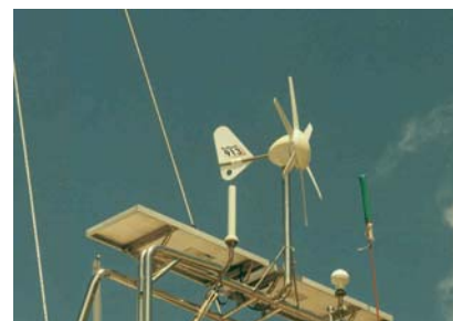
Rutland 913 mounted on a gantry
